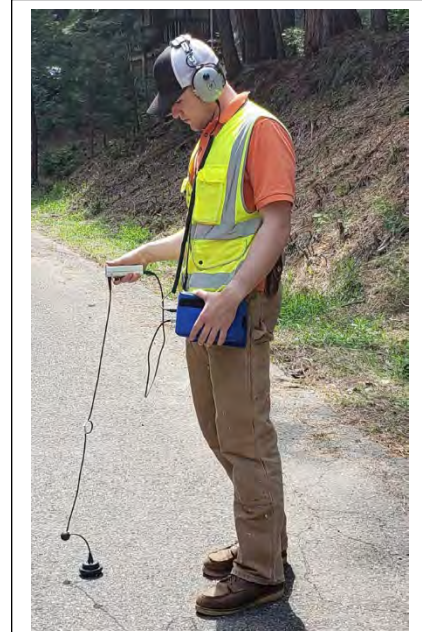
H2Ou Water Operator performing leak detection for GFCSD as part of a Prop 84 Grant for the District. Included the purchase of equipment and performing an entire system survey. H2Ou developed leak program and performed survey.
