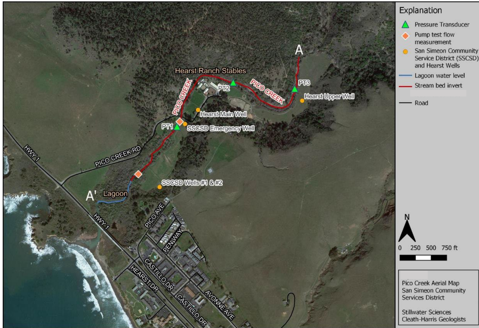
Figure 6. Study Area showing pressure transducer locations (PT1, PT2, and PT3) and pump test stream flow monitoring locations.
