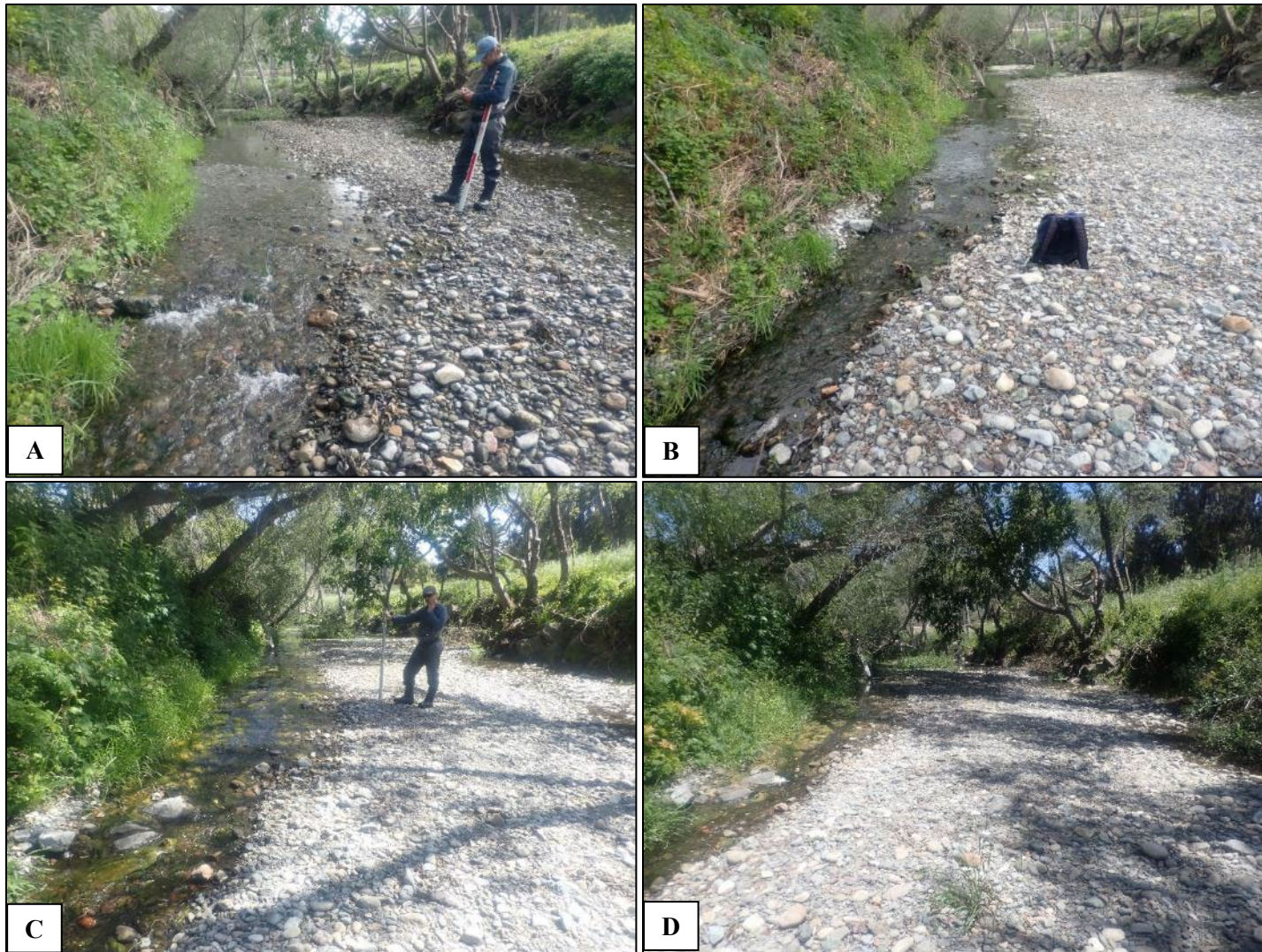
Figure 19. Riffle habitat at PPT1 showing suitable BMI habitat and juvenile steelhead passage at 0.86 cfs (A), BMI habitat but no juvenile steelhead passage at 0.35 cfs (B) and 0.11 cfs (C), and no BMI habitat or juvenile steelhead passage at 0.05 cfs (D).
